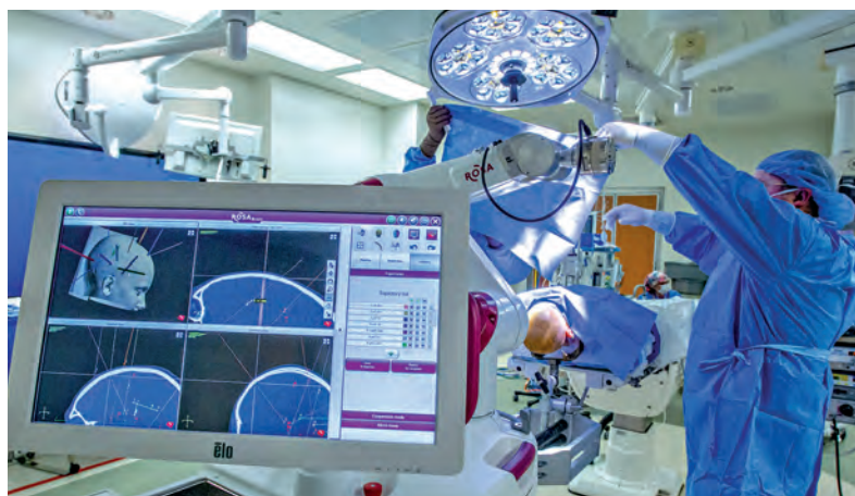
ROSA One Brain's software combines patient imaging to create a 3D map of the patient's brain and head prior to surgery. With this information, neurosurgeons can precisely plan the best placement for electrodes to find seizure areas while avoiding structures critical to function.
