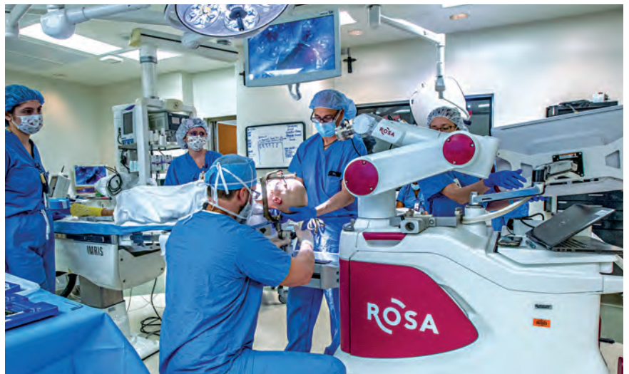
ROSA One Brain's software combines patient imaging to create a 3D map of the patient's brain and head prior to surgery. With this information, neurosurgeons can precisely plan the best placement for electrodes to find seizure areas while avoiding structures critical to function.
